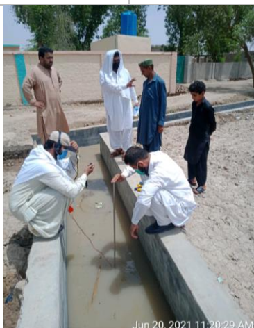
Figure 4.93: Checking Water flow using Pygmy Meter
